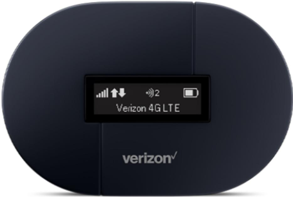
Cellular signal strength, Up/Down arrows, Wi-Fi signal strength, Battery level
